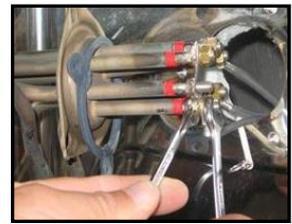
Element electrical connections seen from the rear of the oven
