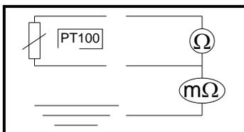
Check sensor resistance with an ohmmeter set to 200 ohms (less than 107 ohms for 20°).
