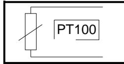
Temperature sensor comprises a resistance sensor with the value of 100 ohms for a temperature of 32°F and 138.5 ohms for a temperature of 212°F. The variation of the resistance to temperature relationship is linear. The resistance reading is directly proportional to the measured temperature. The sensor is not polarised. The sensor can be extended using copper wire.
