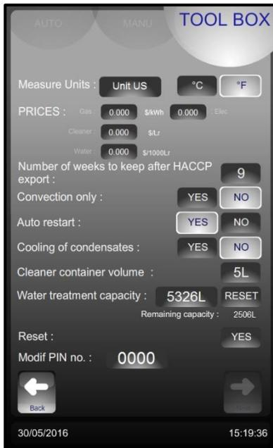
→ The water treatment system's capacity in litres
