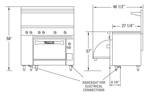
The EV 48 ranges require two separate electrical hook-ups.
